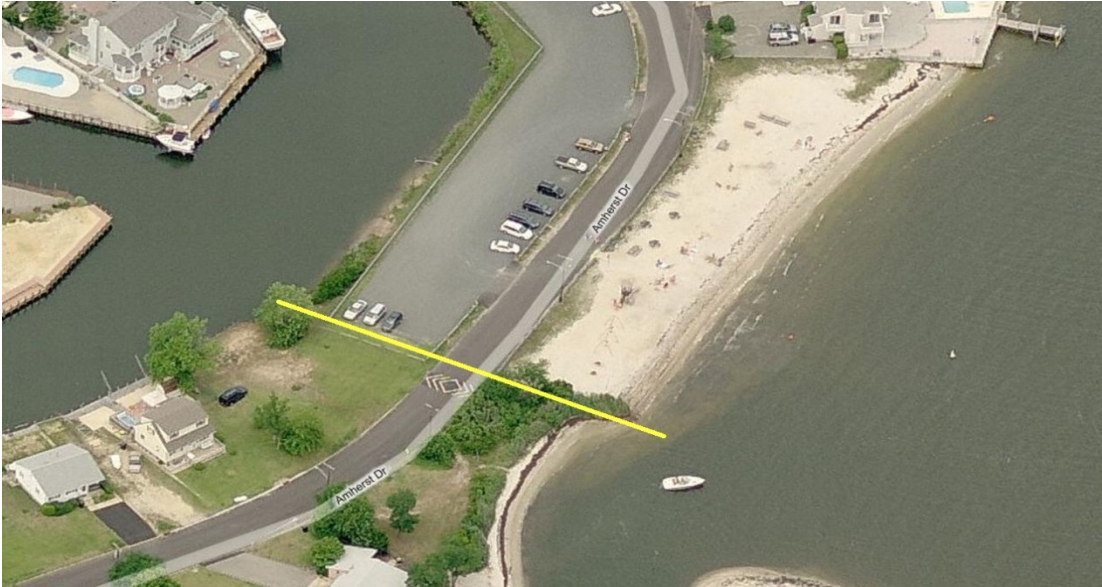
Another possible location for a tidal circulation pipe is between the lagoon on the west side of Amherst Drive and Barnegat Bay at Amherst Beach (recently installed groin not shown).
