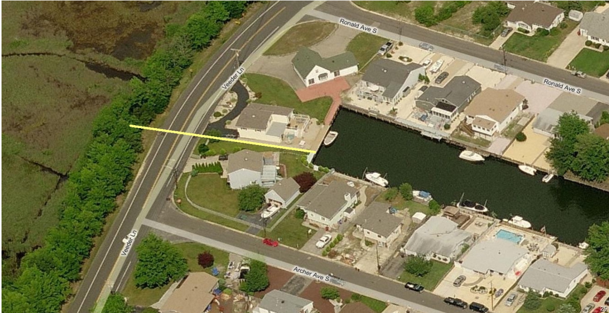
Possible locations for tidal circulation pipes to purify lagoon water
