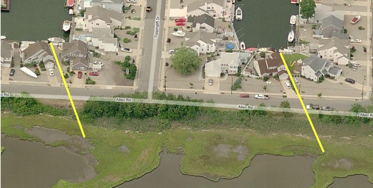
Possible locations for tidal circulation pipes to purify lagoon water
